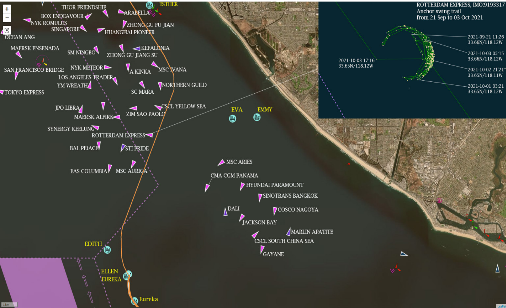
Figure 6 - Rotterdam Express plotted track in anchorage with no sign of dragging anchor, 03 rd October 2021
